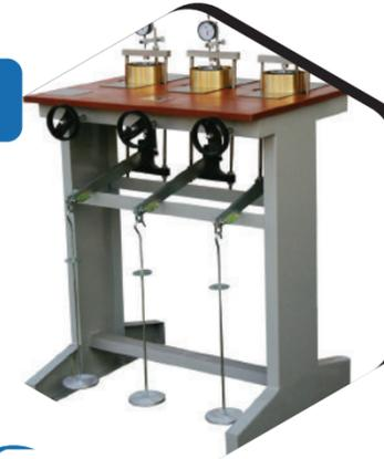
Machine de test triaxial
